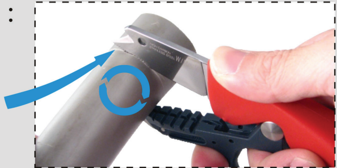
Operate the blade guards with the middle finger
