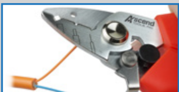
Strip 250 micron cladding down to 125 micron bare fiber
